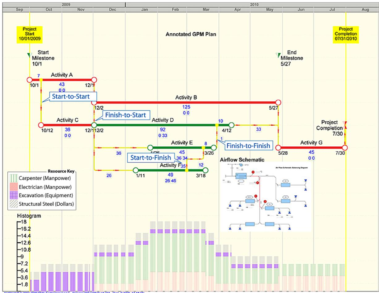
Figure 3 Annotated Graphical Path Method, Logic Diagram Method (LDM) diagram <sup>8</sup>
